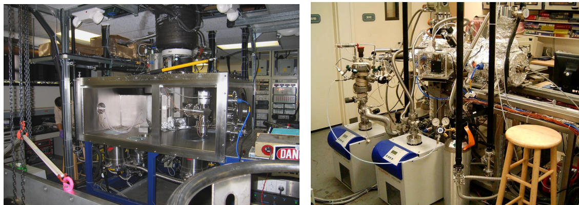
Figure 1: Images of the crossed molecular beams machine (left) and the surface scattering machine (right) utilized to study bimolecular neutral-neutral reactions in the gas phase and the interaction of ionizing radiation with (icy) surfaces.
